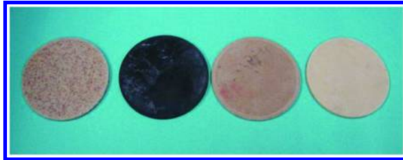
Figure 12. Optical photograph of rubber samples with 15% soy meal, 15% carbon black, 15% soy flour, and no filler (from Left to Right.)
