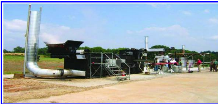
Figure 2. NCSU Continuous Self-Fueling Prototype Torrefactor. Reproduced with permission from Reference (23). Copyright [2014] [Agri-Tech Producers, LLC].
