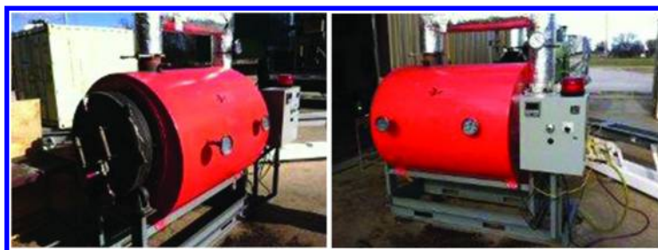
Figure 4. ECP Prototype Pilot Torrefactor. Reproduced by permission from Reference (24). Copyright [2014] [Greg Karr].
