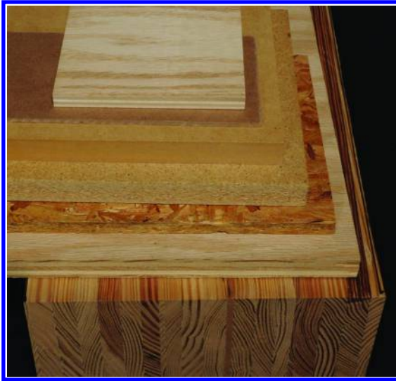
Figure 1. Some wood products from top to bottom, engineered wood flooring (soy), hardboard, fiberboard (UF), particleboard (UF-soy), OSB (soy-PF), interior plywood (soy), glulam (casein).
